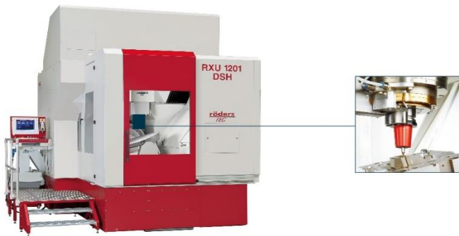
Image: Rödgers milling machine with integrated medium distributor via a spindle adaptation
