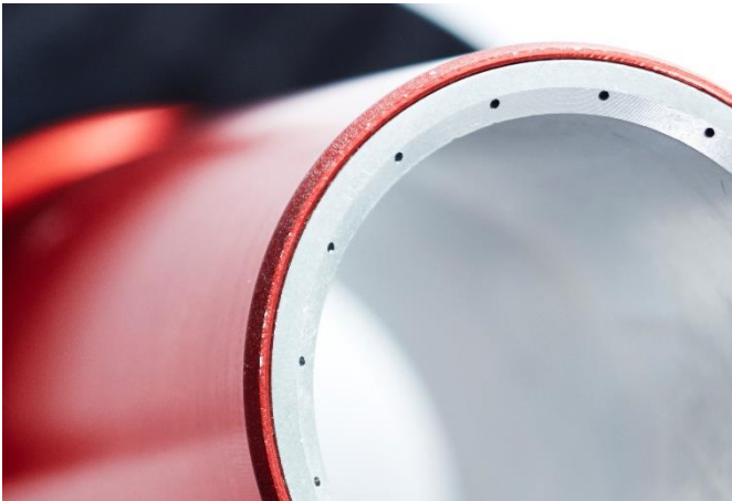
Image: Nozzle, fine oblique holes of 0.5mm ensure a constant air jet and a high flow velocity
