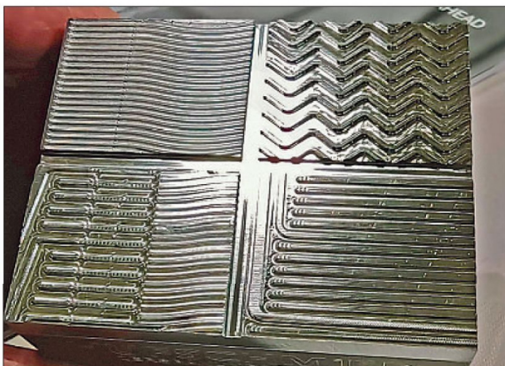
Sample workpiece (50 x 40 mm) with various surface structures typical of bipolar plates (photo: Klaus Vollrath)
