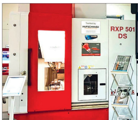
The demonstrator was milled in Hufschmied's technical center on this five-axis Rödgers RXP 501 DS; the system is equipped with the MHT medium distributor (photo: Klaus Vollrath)
